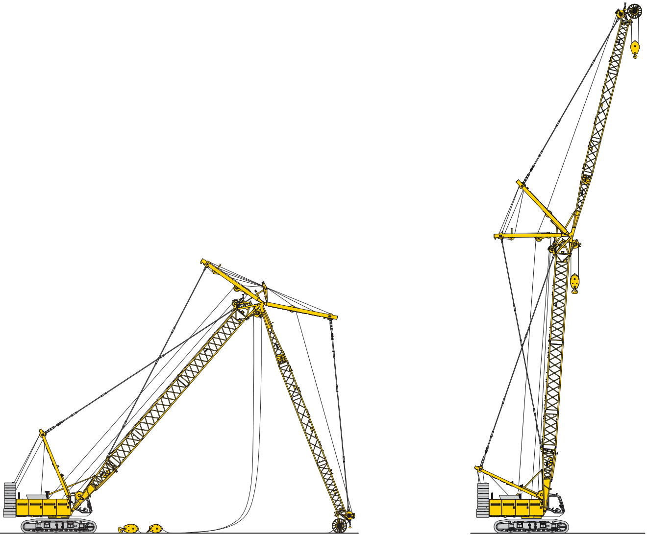
Erecting of main boom and luffing jib
