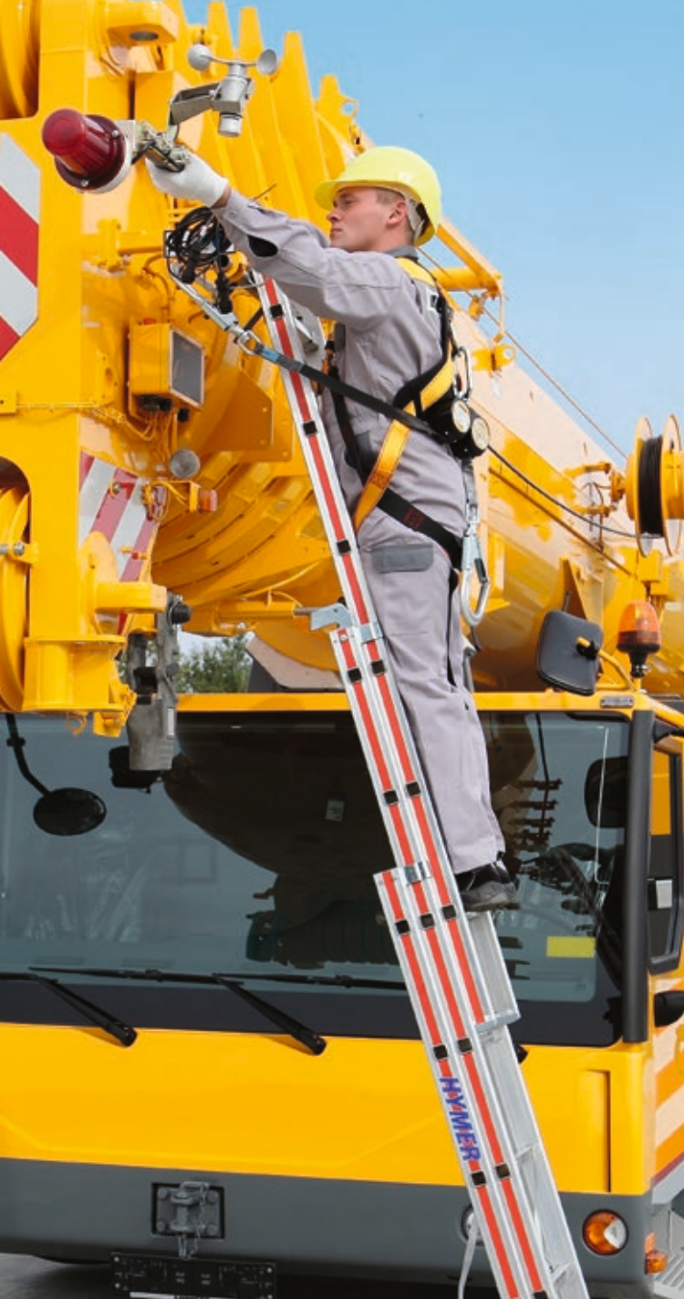
Special holder at the crane for safe positioning of the ladder
