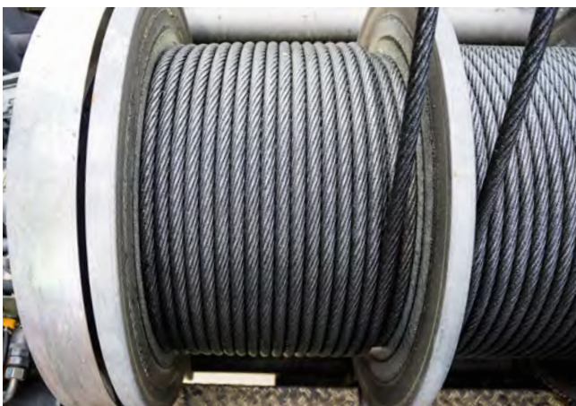
Hoist rope perfectly coiled
