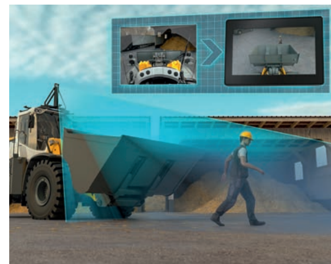
Liebherr presents a complete package of driver assistance systems at Bauma: the active rear-view human detection system, frontal area monitoring and the SkyView system ensure even greater safety on the construction site. The new joystick steering system, the tyre pressure monitoring system and Liebherr’s own weighing system with Truck Payload Assist increase the efficiency of the wheel loaders
