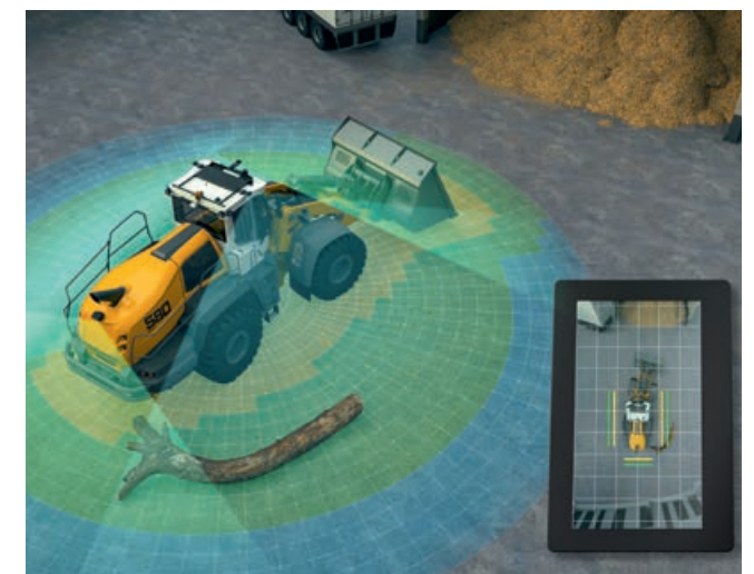
Liebherr presents a complete package of driver assistance systems at Bauma: the active rear-view human detection system, frontal area monitoring and the SkyView system ensure even greater safety on the construction site. The new joystick steering system, the tyre pressure monitoring system and Liebherr’s own weighing system with Truck Payload Assist increase the efficiency of the wheel loaders
