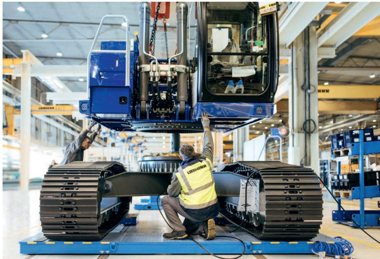
A special union: the undercarriage and uppercarriage of the 60,000th crawler excavator are mounted
