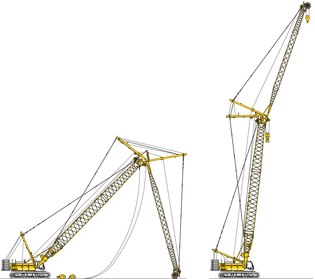
Erecting of main boom and luffing jib
