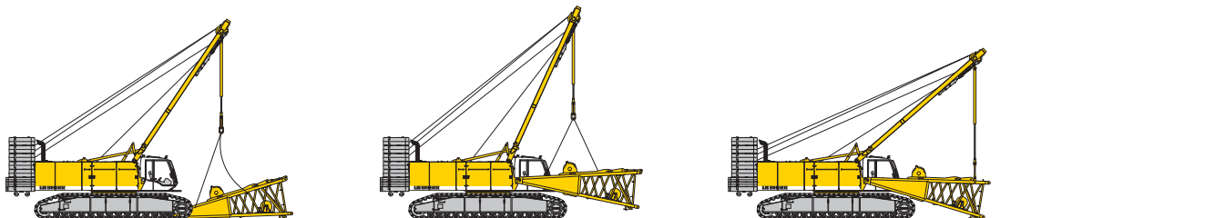
Unloading and assembly of boom foot
