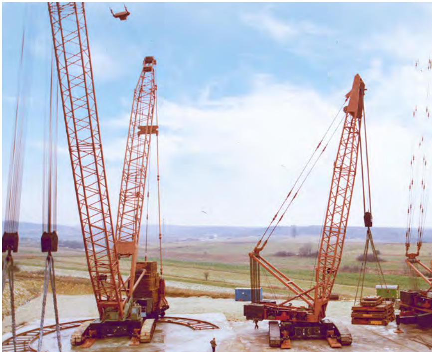
On the Liebherr test site in Ehingen in 1977 – LR 1300 with and without derrick system.
