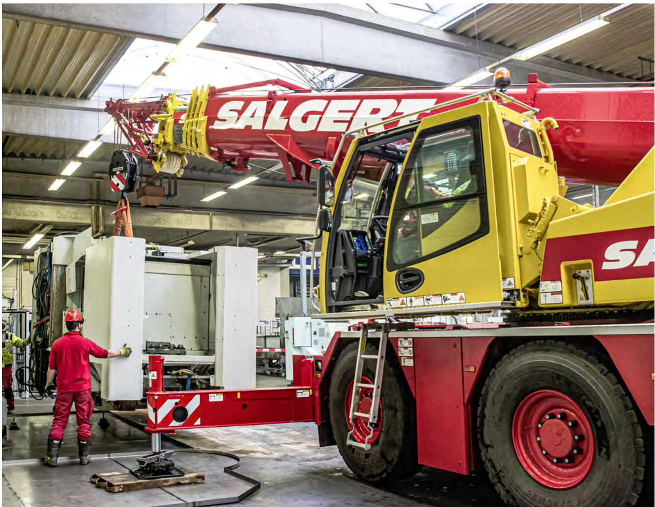
Top work – the special erection jib on the LTC 1050-3.1 enables maximum hoisting height to be used in low buildings.
