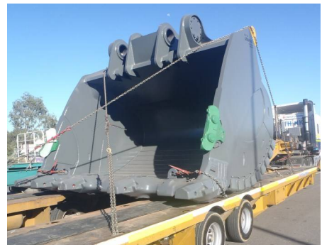
An Adelaide-fabricated R 996 bucket, destined for export to Chile. ►
