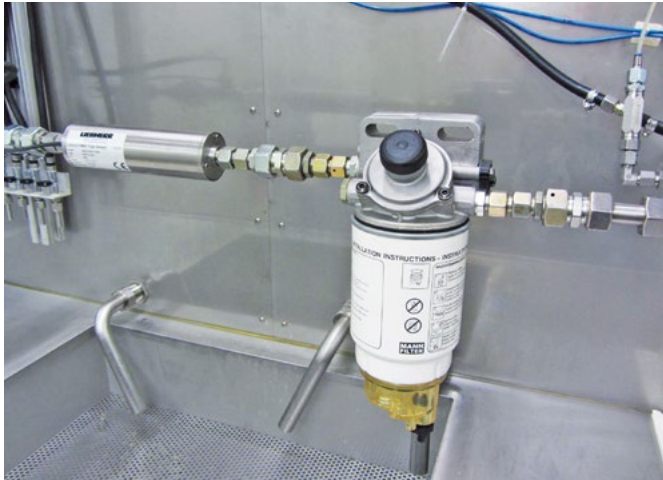
Litronic-FMS / RMH12 sensor integrated in a test and a laboratory plant to monitor the demulsification capacity of a diesel fuel filter.
