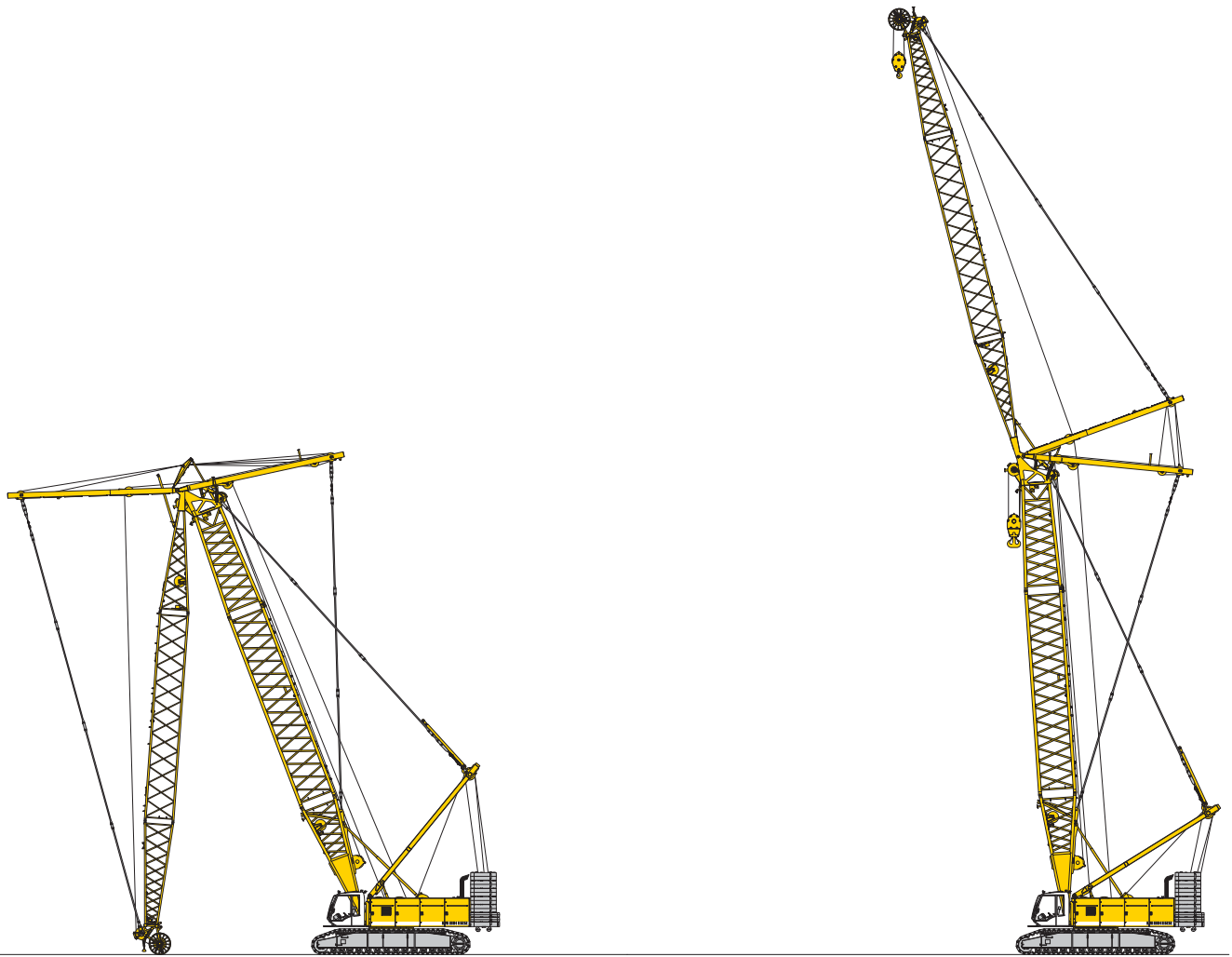
Erecting of main boom and luffing jib
