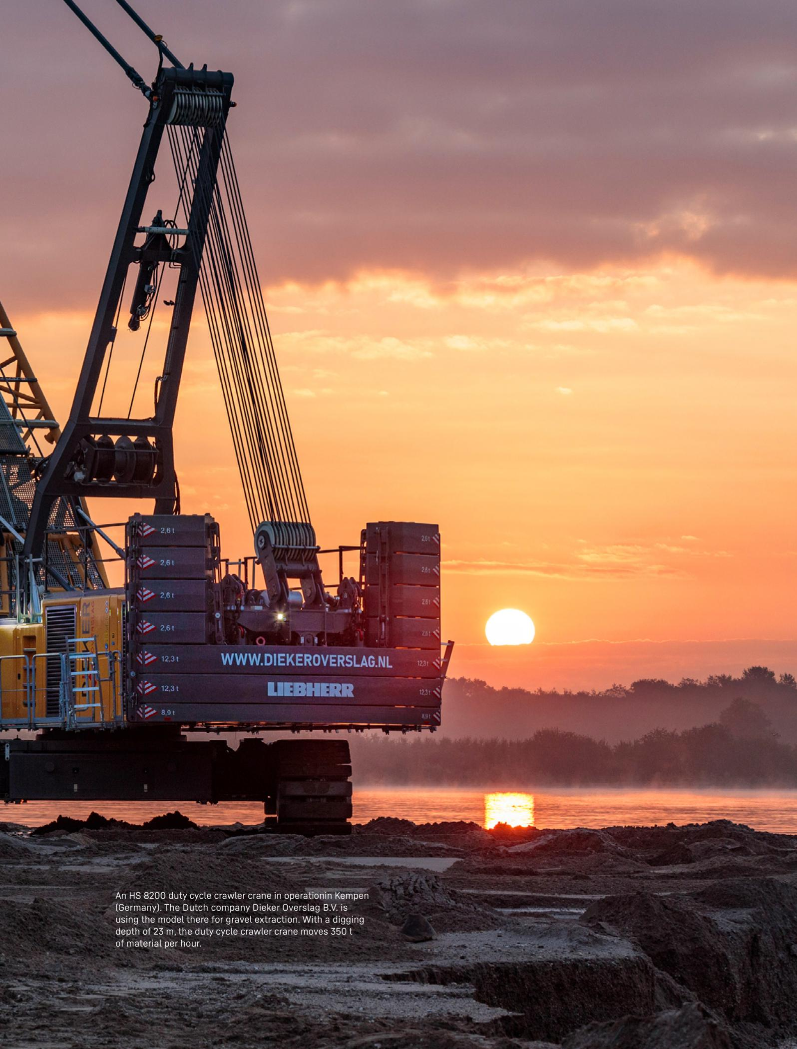
An HS 8200 duty cycle crawler crane in operation in Kempen (Germany). The Dutch company Dieker Overslag B.V. is using the model there for gravel extraction. With a digging depth of 23 m, the duty cycle crawler crane moves 350 t of material per hour.
