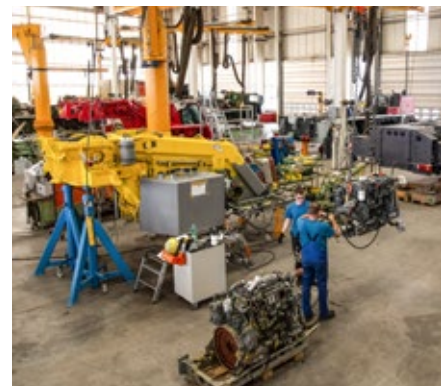
Replacement of the superstructure engine and repair of the turntable
