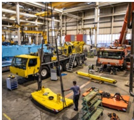
Complete dismantling of the crane
