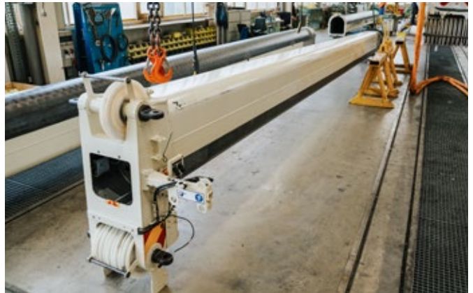
Reconditioning of a telescopic boom
