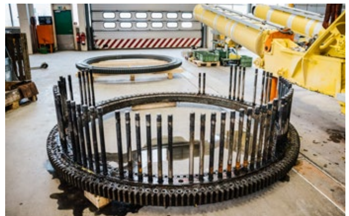
Slewing ring inspection with subsequent replacement
