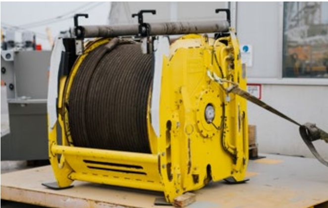
Hoist rope and winch inspection for the check to meet accident prevention regulations under §26 BGV D6
