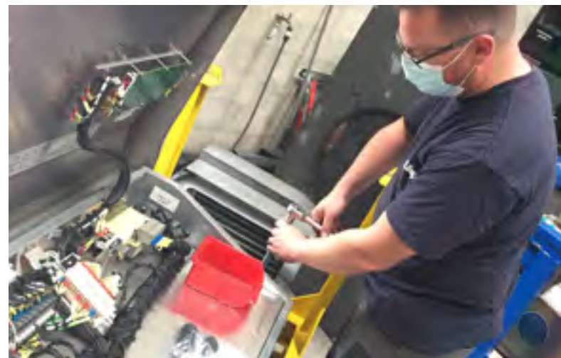
Overhaul of an air-conditioning unit
