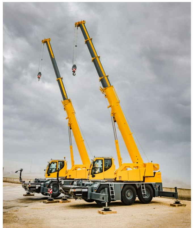
LTC 1050-3.1 with TELEMATIK boom and with rope pull mechanism (right)
