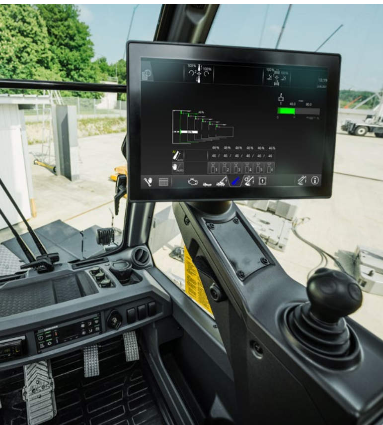
Display with touchscreen function in the superstructure cab ensures intuitive, convenient control
