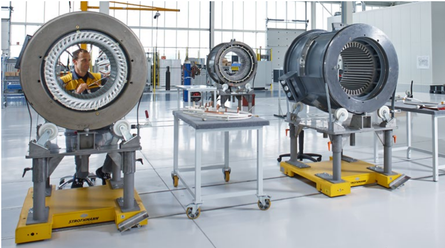
Winding of electric machines for mining trucks and port cranes
