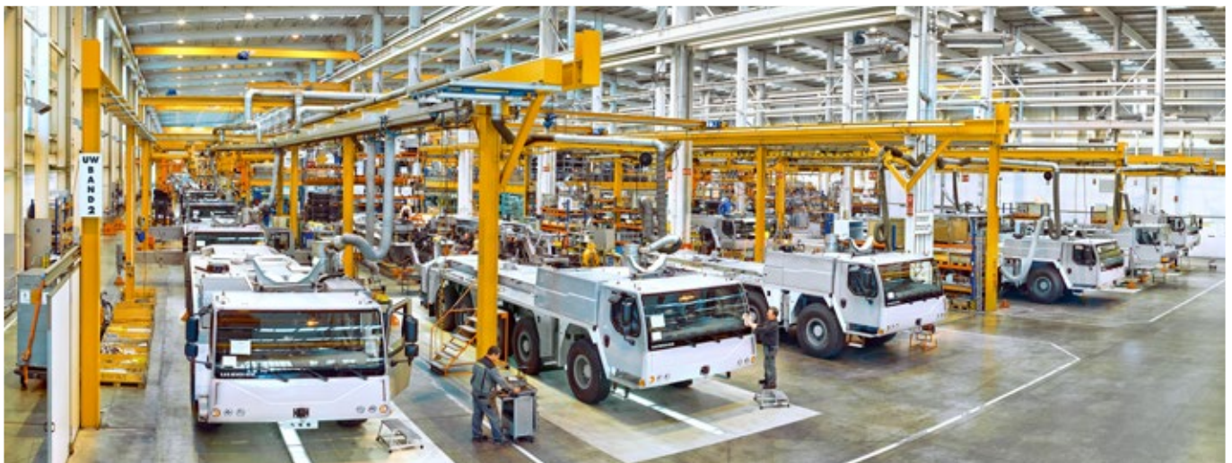
Final assembly of the mobile cranes in the Liebherr plant in Ehingen (Germany)
