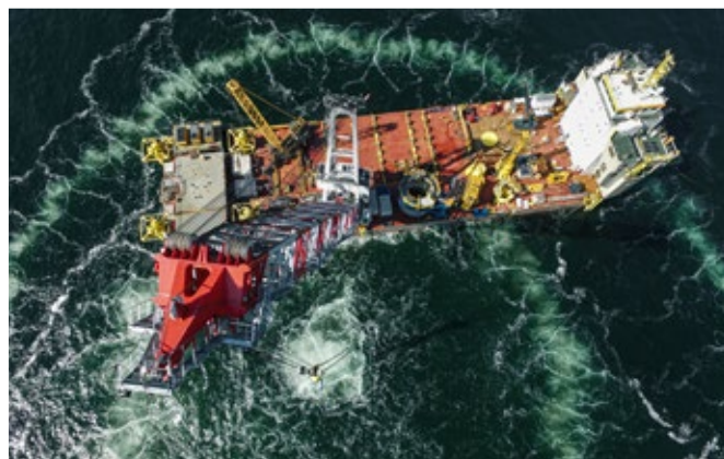
With a maximum lifting capacity of 1,250 tonnes, the board offshore crane BOS 35000 is designed to handle heavy and large components
