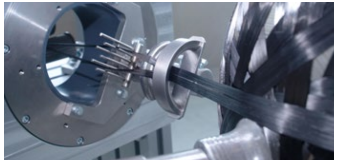
CRP production using the in-house robotised winding machine
