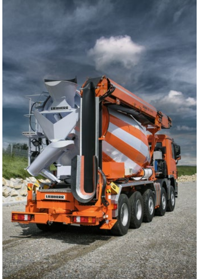
The truck mixer HTM 1004 with double telescopic conveyor LTB 12+4+1
