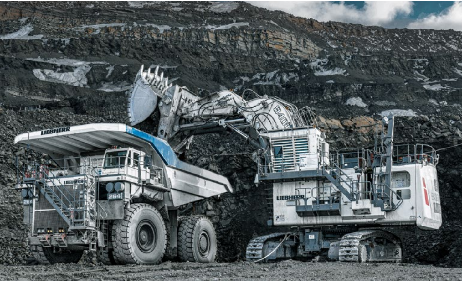
Liebherr R 9400 loading a Liebherr T 264 truck
