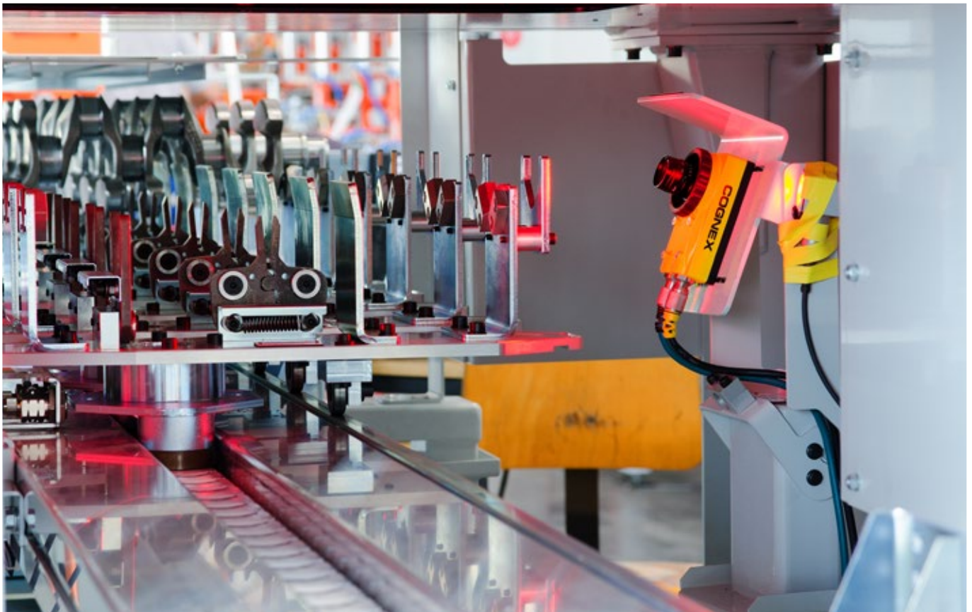
The plastic chain conveyor (KKB) as conveying system for crankshafts for example
