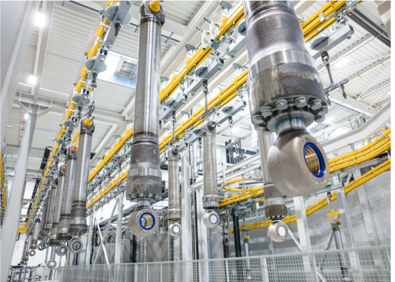
Robotised coating line for hydraulic cylinder series-production ranges
