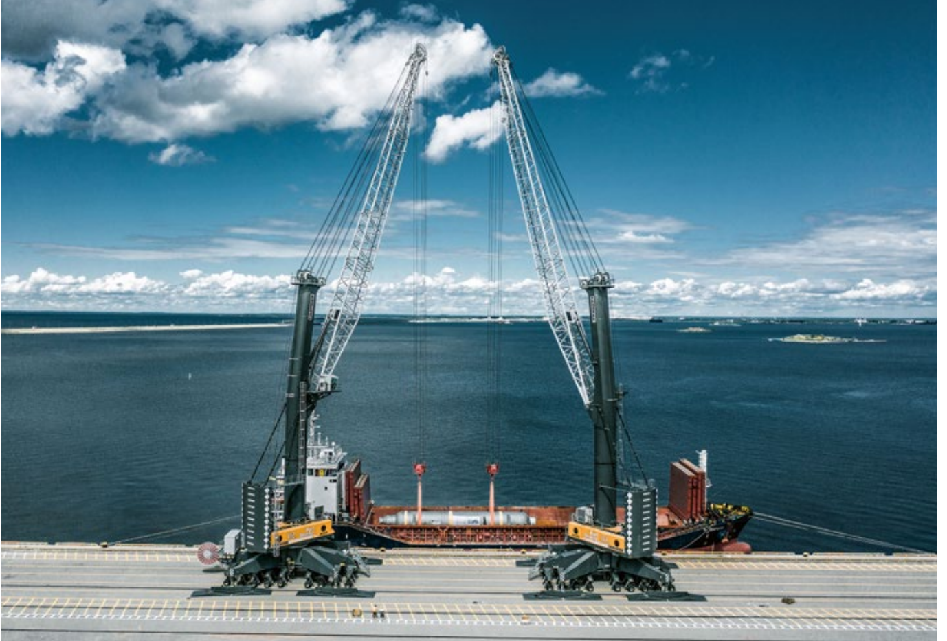
Two mobile harbour cranes LHM 800 in tandem lift operation at the Port of Saint-Petersburg (Russia)
