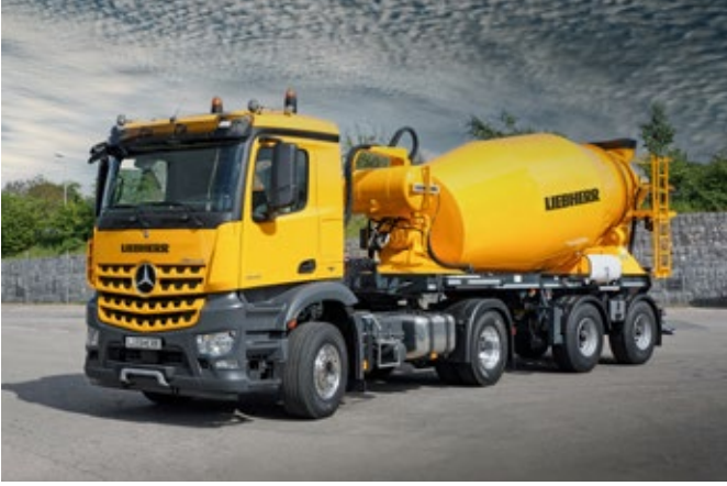
The truck mixer HTM 1004 ZA/38 is approved for a total weight of 38 t
