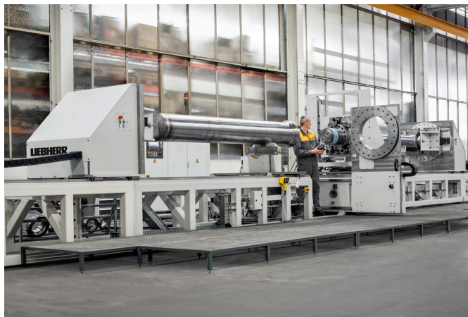
Mining cylinder assembly line Designed by Liebherr to assemble heavy duty cylinders in highest precision
