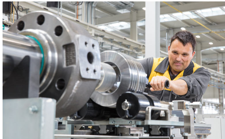
Piston rod assembly line Assembly of piston to rod with automatized process inclusive torque controll
