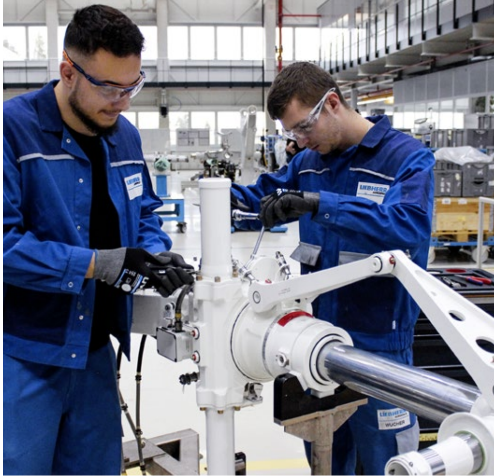
Assembly of an overhauled landing gear at the Liebherr-Aerospace facility in Lindenberg (Germany)
