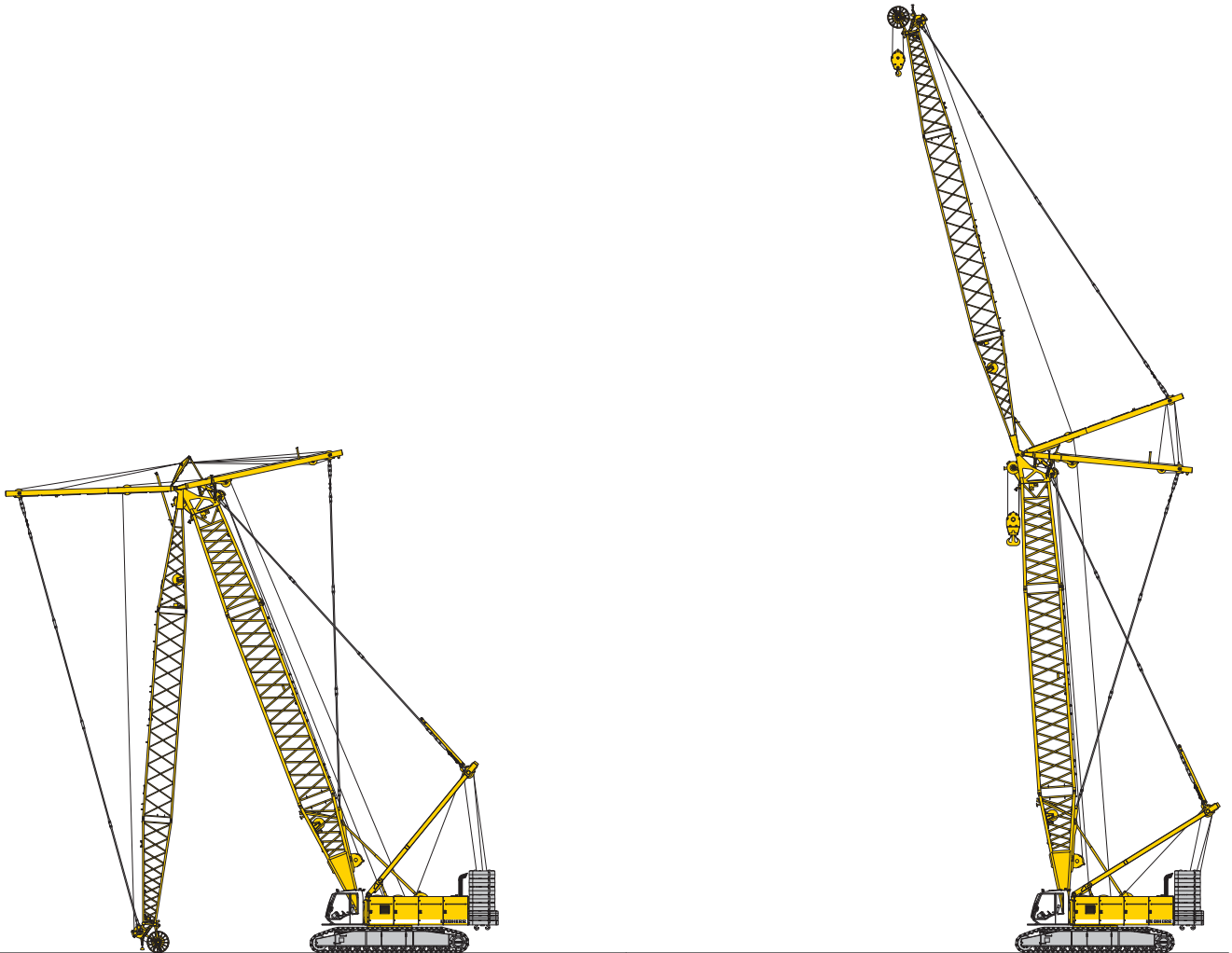
Erecting of main boom and luffing jib
