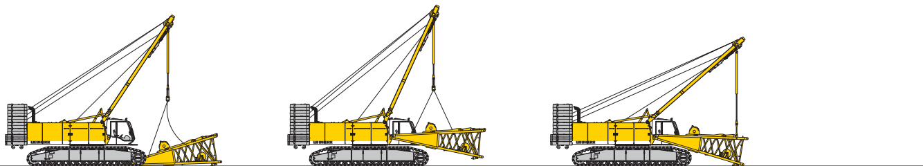
Unloading and assembly of boom foot
