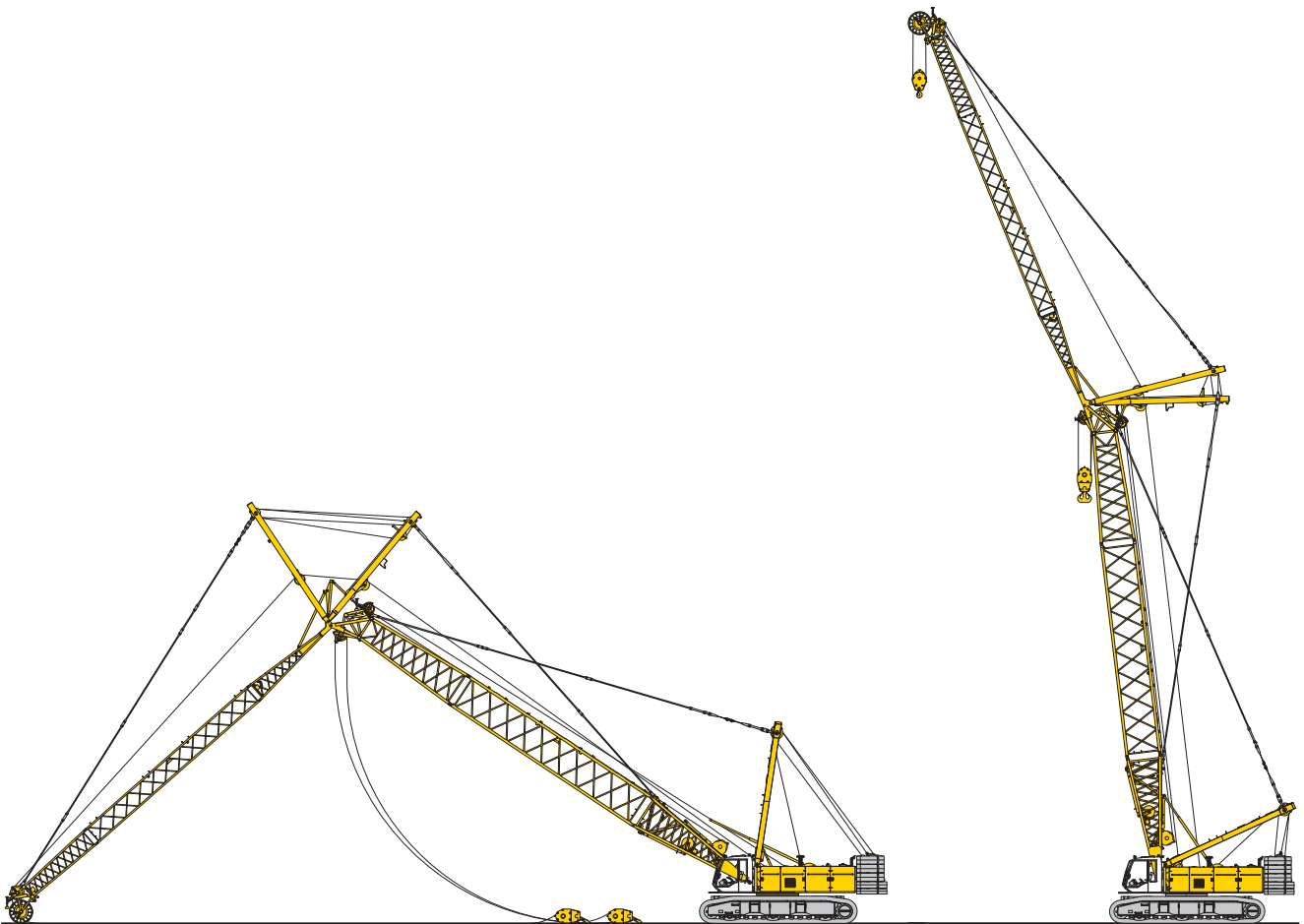
Erecting of main boom and luffing jib
