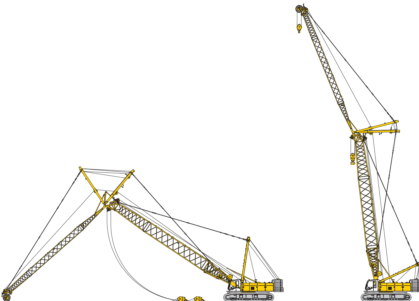
Erecting of main boom and luffing jib
