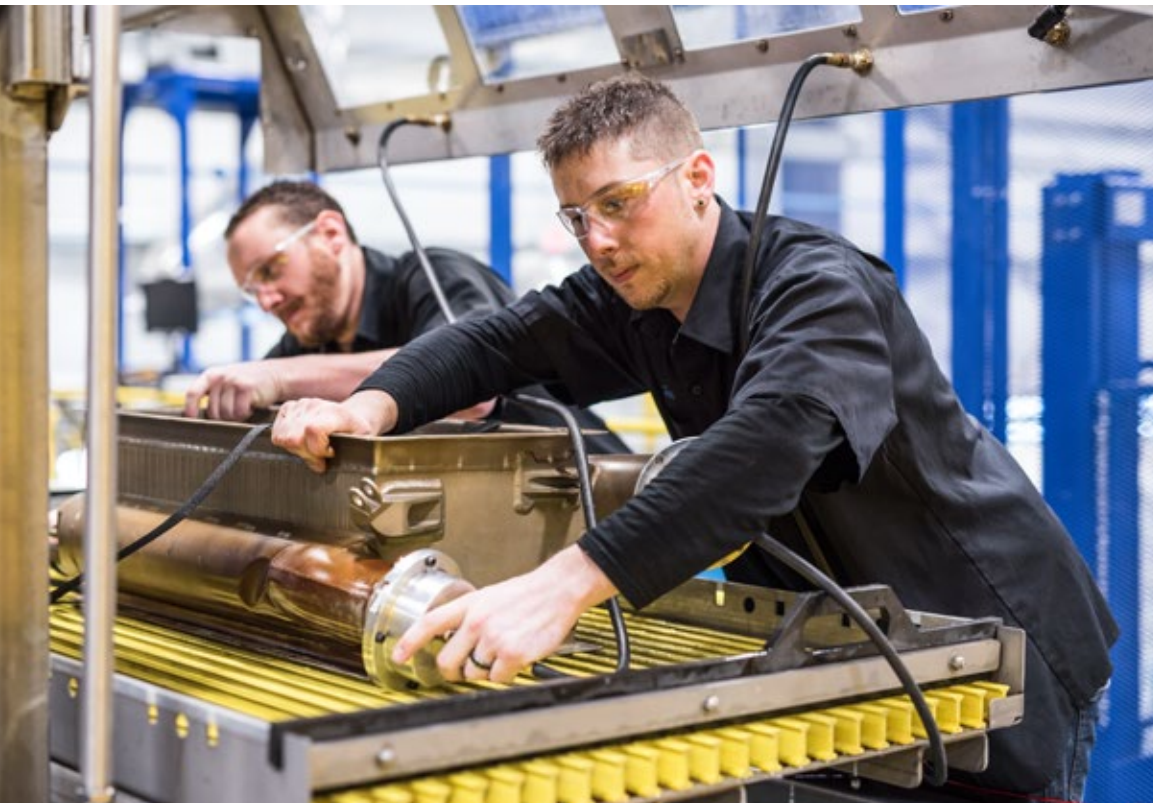
After cleaning, the heat exchanger is tested.
