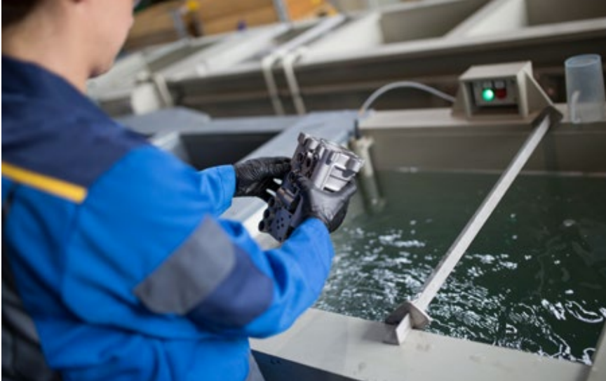
To remove powder residues from the components reliably, they are cleaned in an electro-chemical bath in Lindenberg after manufacture.
