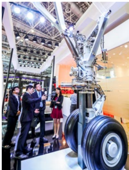
Airbus A350 XWB Nose Landing Gear
