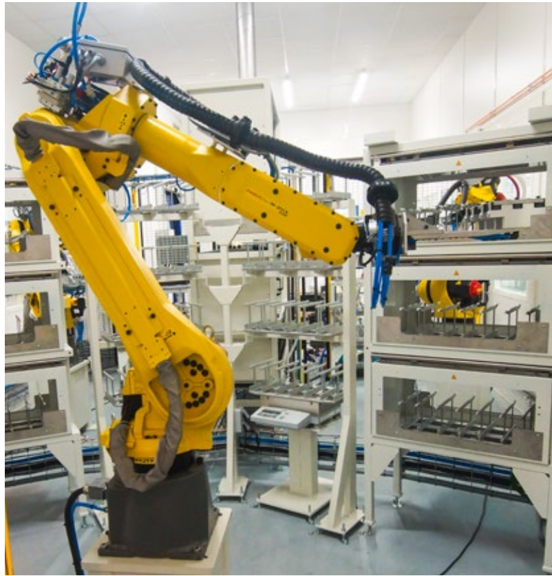
Four robots in total are used at Liebherr-Aerospace in Toulouse in the heat exchanger manufacturing process. The robot responsible for handling takes the individual separator plates for processing.
