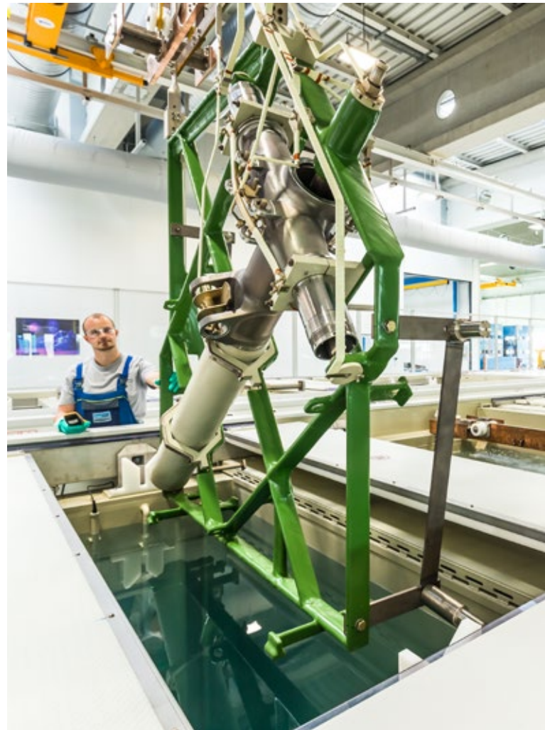
With the new zinc-nickel coating plant, Liebherr-Aerospace is now also able to coat large components itself.
