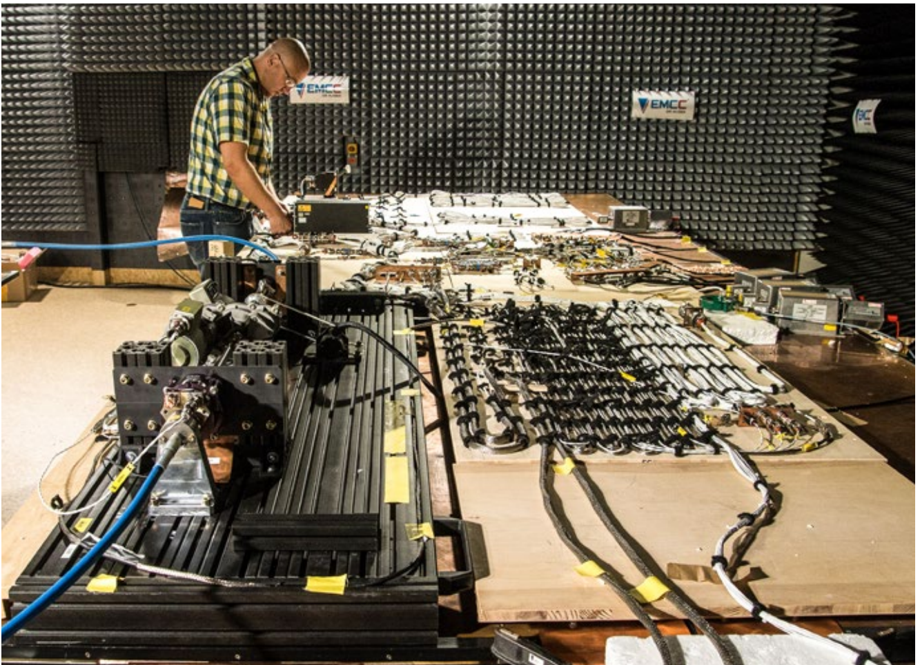
In order to ensure interference resistance to electromagnetic fields, all components of the flap/slat control system in the new E-Jet E190-E2 were tested in the EMT laboratory for three months.
