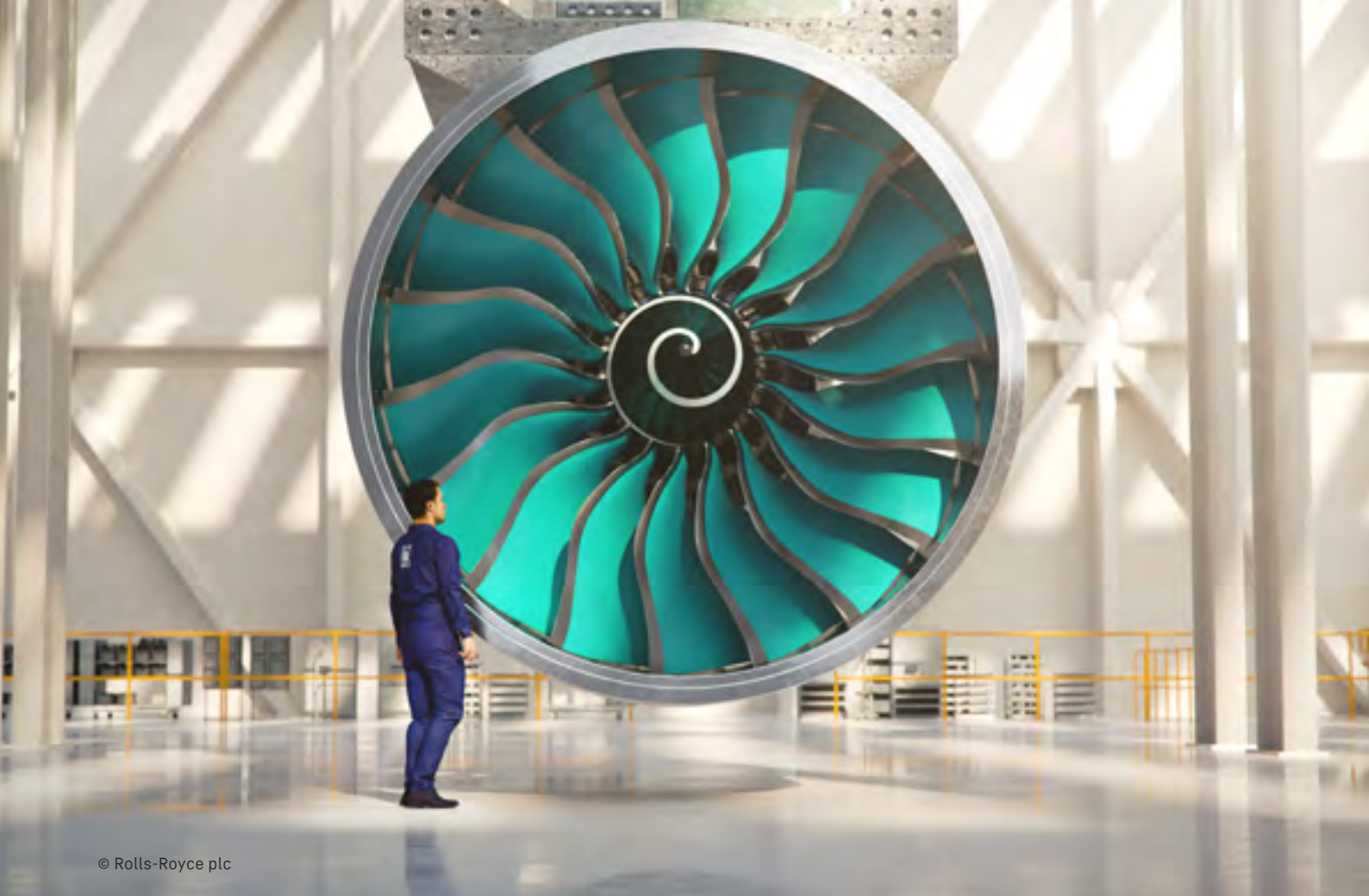
Carbon fiber composite and titanium fan set with a diameter of more than 3.50 meters (140 inches)
