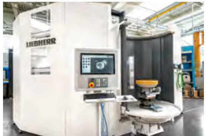
The new high-capacity five-axis machining center with a Rotary Loading System at Liebherr-Aerospace in Campsas
