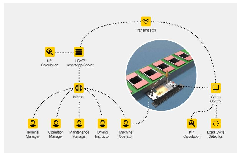
The relevant data generated and preprocessed by the crane control system during operation are transmitted by the established LiDAT® Technology to the LiDAT® smartApp server to be stored and preprocessed. Authorised users can access and download the processed data via LiDAT® smartApp, a software solution which is designed as web application. Liebherr handles the setup and support of the transmission link, hosts the data and maintains the software during the active user subscription.
