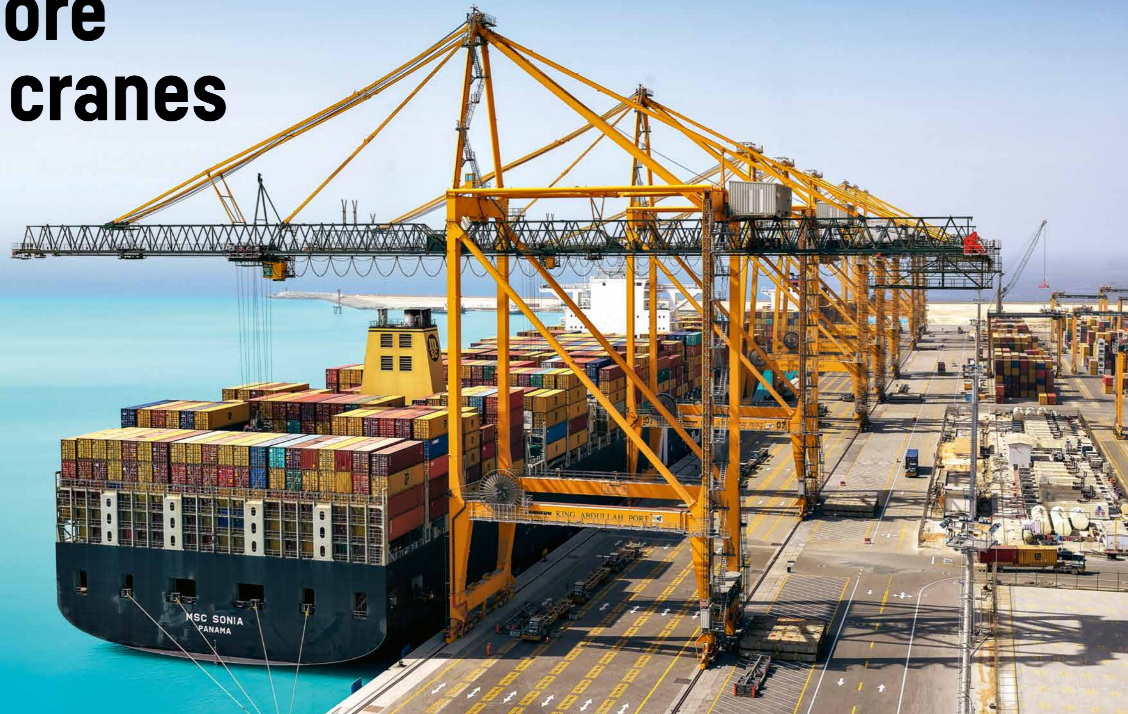
Liebherr Megamax STS cranes working an ultra large container vessel in Saudi Arabia
