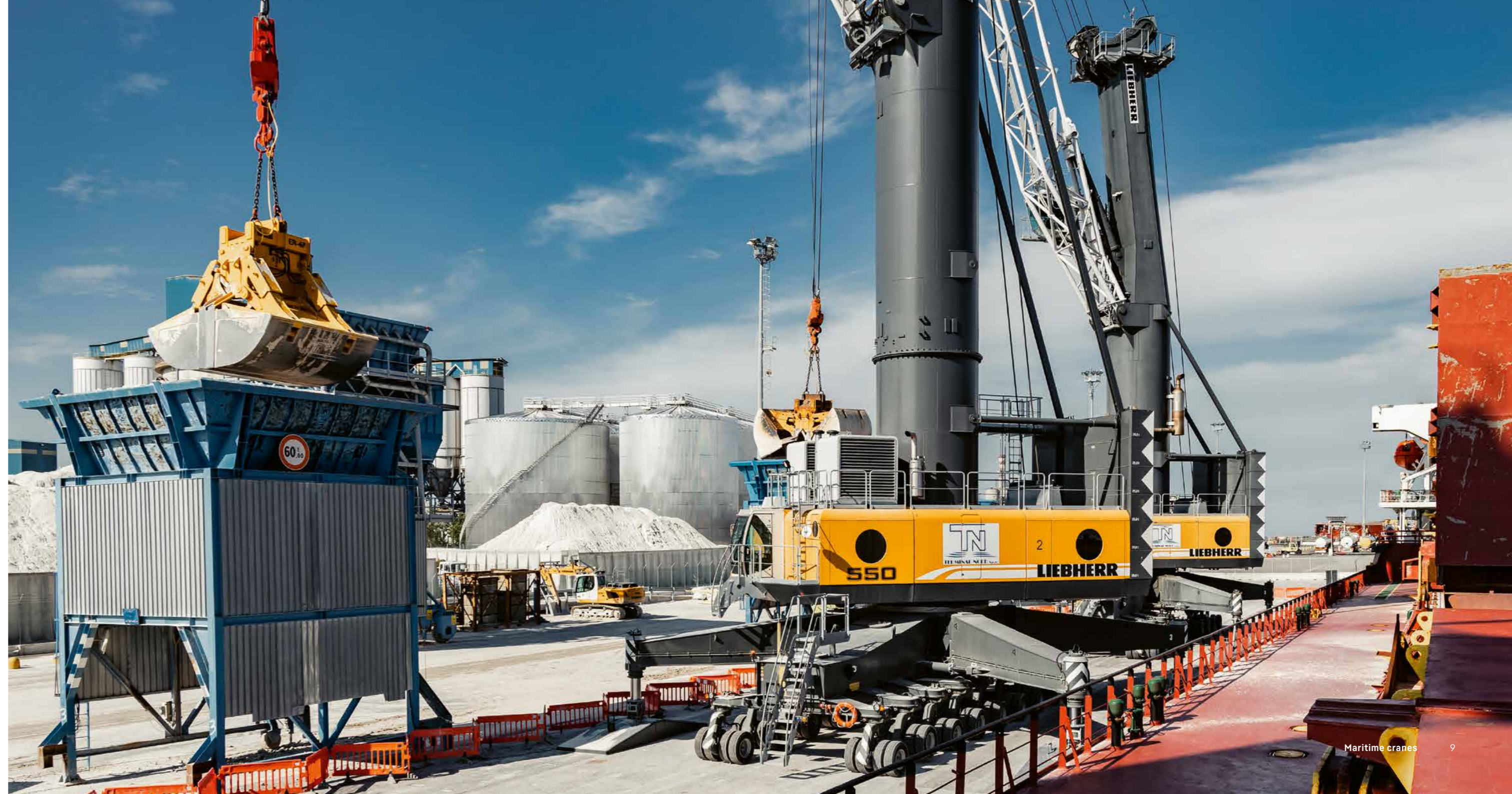
Liebherr mobile harbour crane type LHM 550 handling clay in Italy
