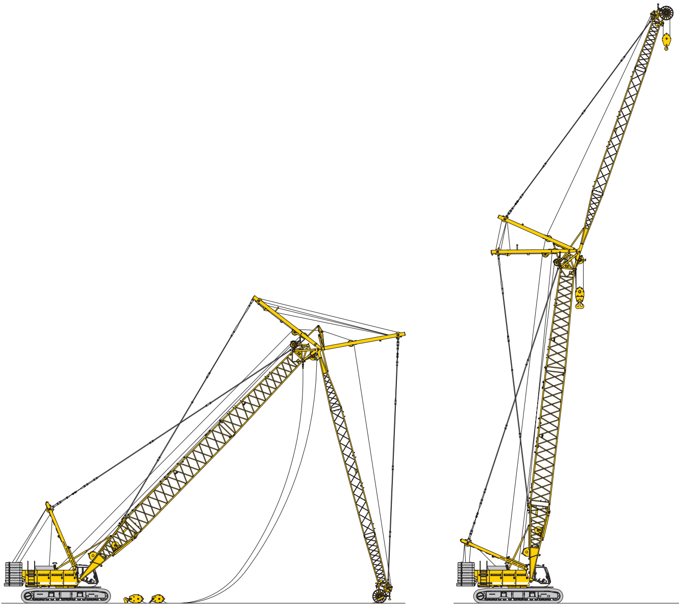
Erecting of main boom and luffing jib
