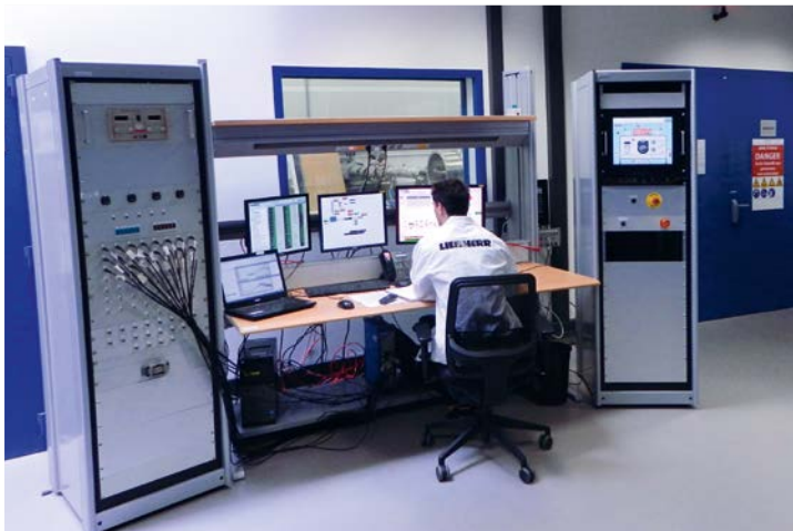
Anechoic chamber monitoring and control system
