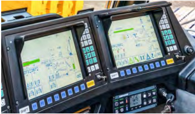
The systems send all the parameters for the crane status and hoisting process to the operator's cab of the R 1700-1.0. The right-hand display shows a current load case of 86 tonnes.
