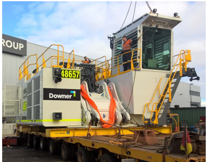
Downer's R 9400, ready for transport to site.
