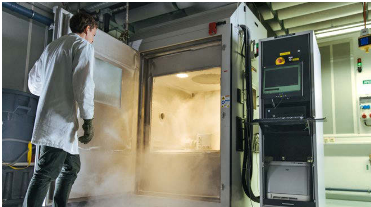
In the Liebherr Test Centre for electronics, components are stressed to test their performance
