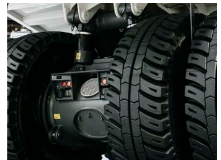
Service door on axle box for inspections
