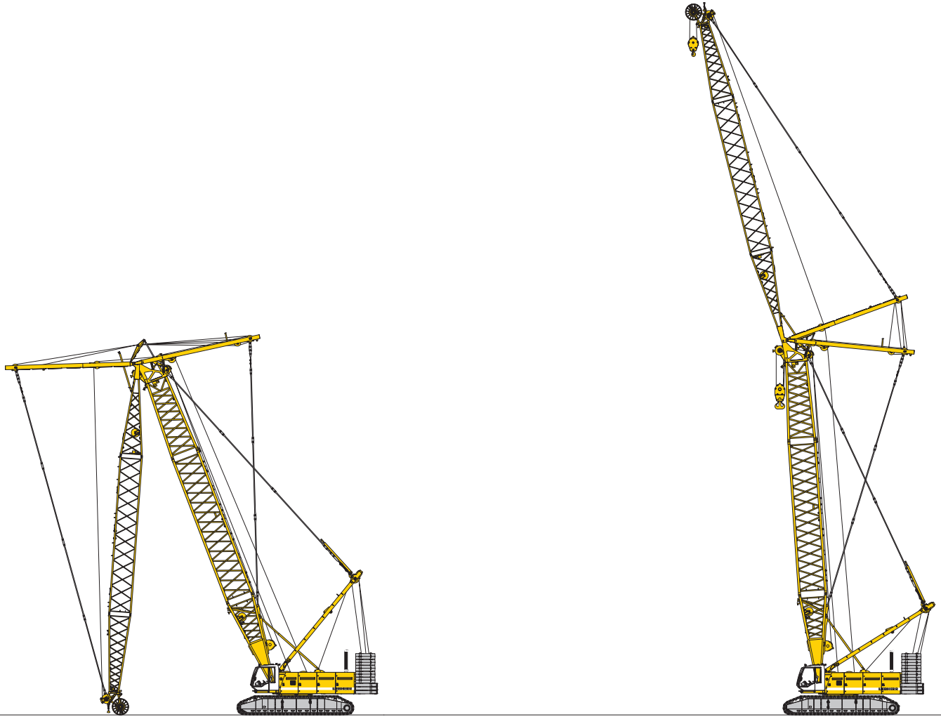
Erecting of main boom and luffing jib
