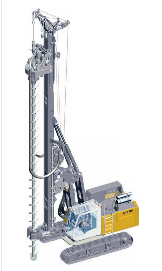
Auger with auger guide
