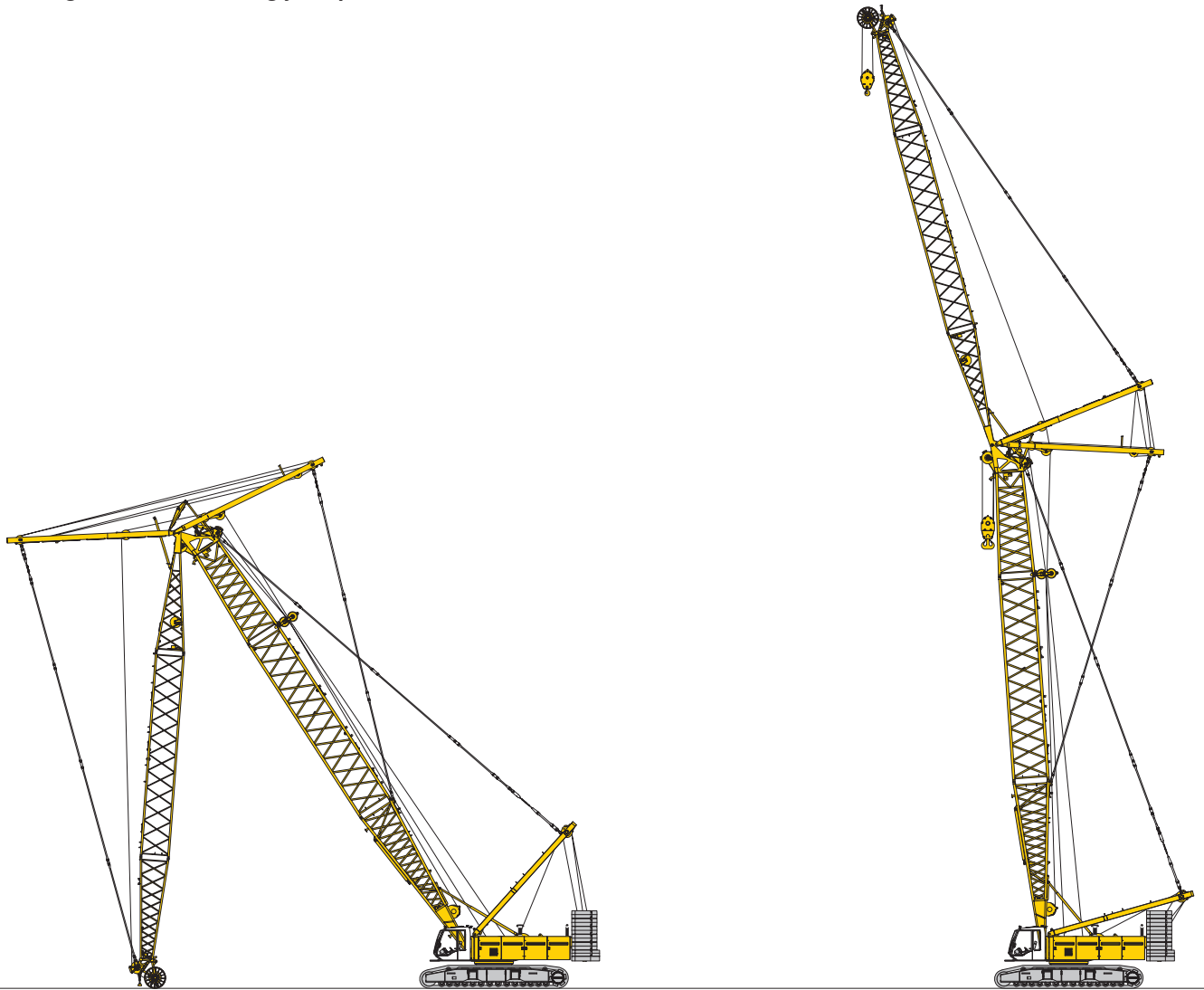
Erecting of main boom and luffing jib
