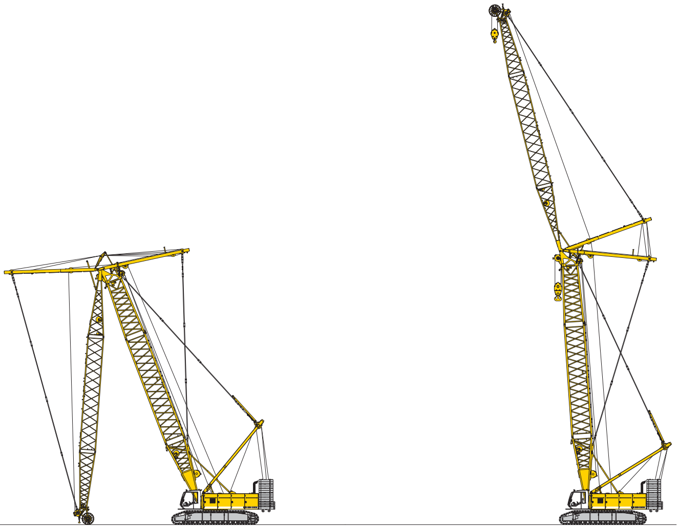
Erecting of main boom and luffing jib
