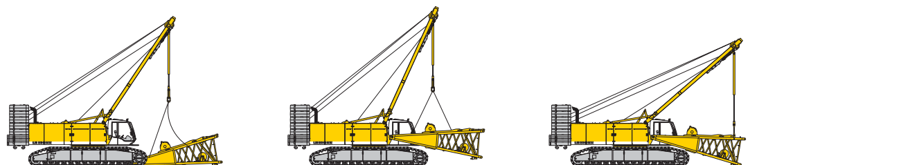
Unloading and assembly of boom foot
