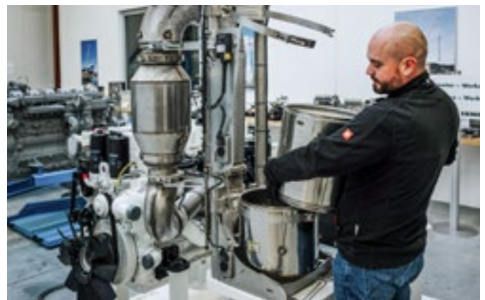
Trainer Thomas Fritsch demonstrates the replacement of a diesel particulate filter on a model at the Liebherr training centre in Ehingen.
