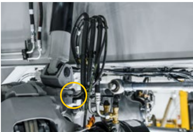
Optimally lubricated Steering knuckles with lubrication line.
