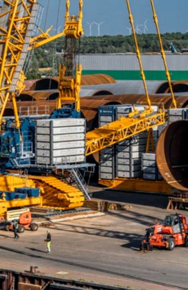
The innovative slewing platform design of the LR 12500-1.0 with its 7.5 metre wide HighPerformanceBoom.
