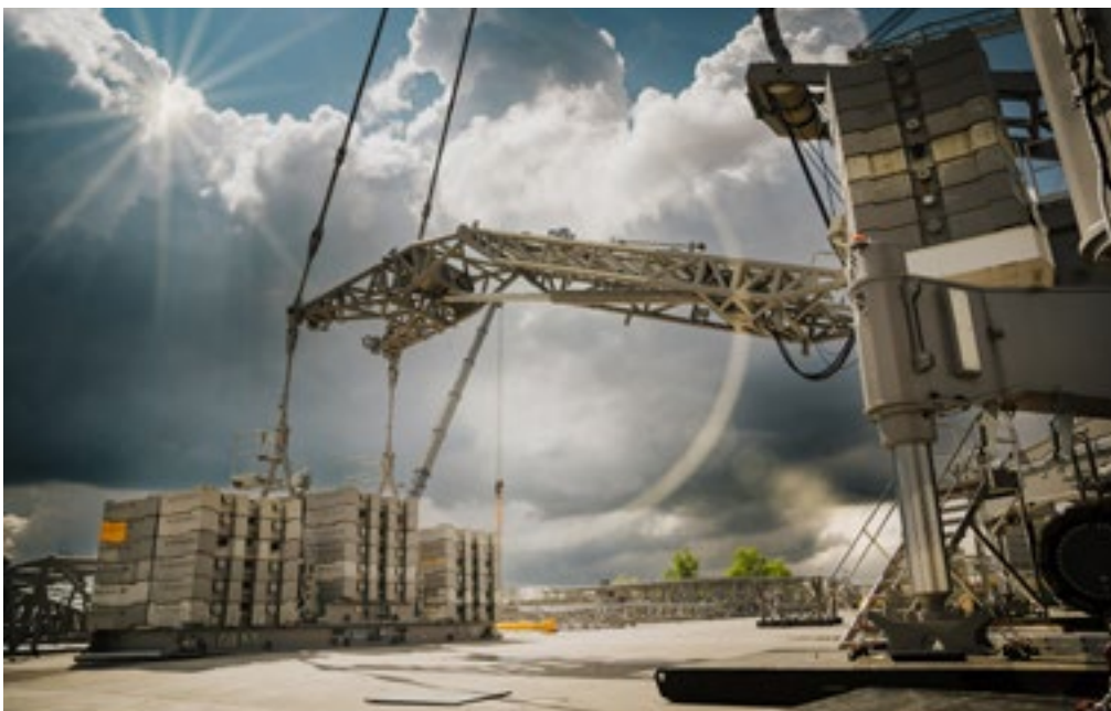
The narrow track version also uses the hydraulically adjustable V-Frame® ballast guide.
