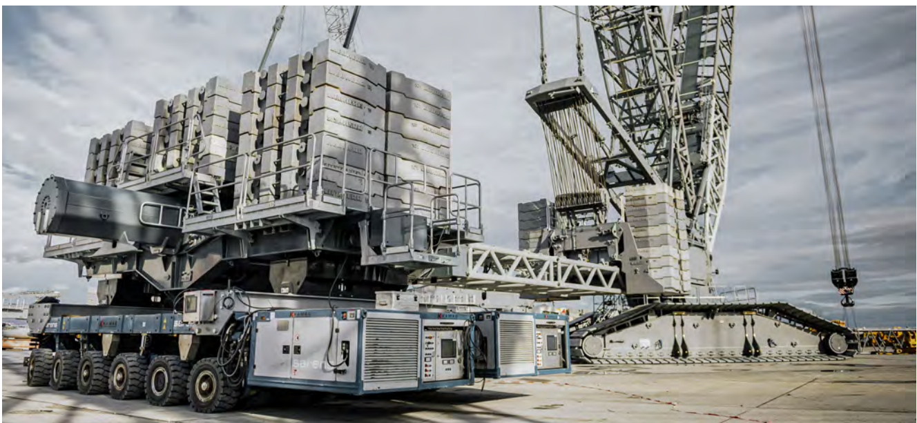
The future – a ballast trailer with an SPMT acting as the undercarriage.
