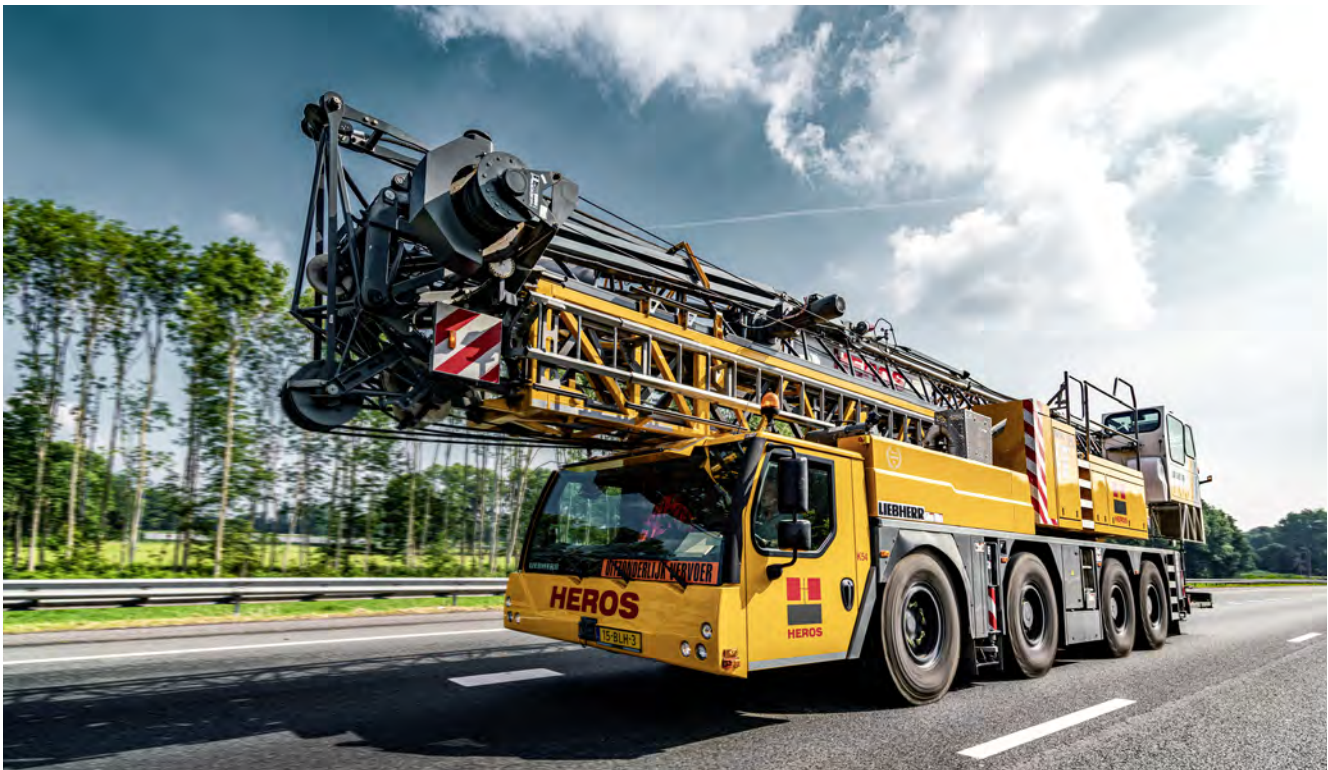
An MK 88 Plus mobile construction crane owned by our customer Heros.
