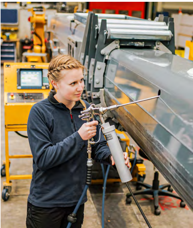
The grease spraying rod can be used to grease the telescopic boom both internally and externally.
