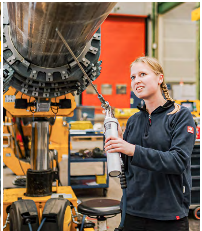
The grease spraying rod can be used to grease the telescopic boom both internally and externally.
