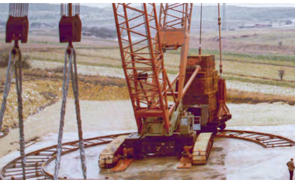
Ballast trailer development at a glance – first on rails, then on tyres.
