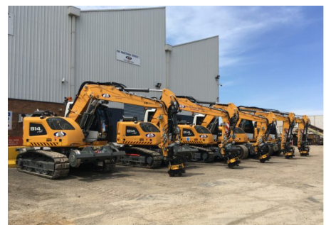
RMS' Liebherr Rail Excavator fleet: 3 x R 914 Rail Excavator (tracked) and 3 x A 922 Railroader (wheeled)
