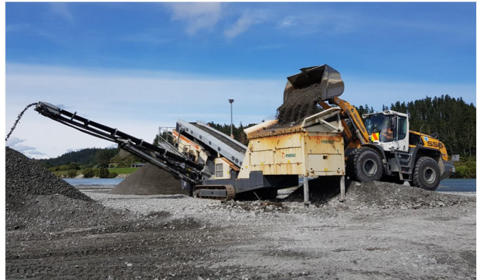
L 550 XPower® Wheel Loader feeding mobile screen at Hokitika River Bed in NZ.
