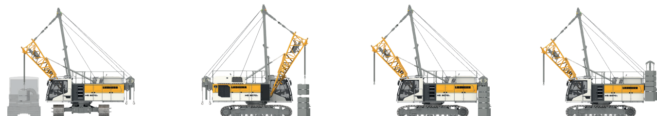
Unloading and assembly of rear counterweight
