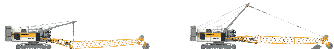
Assembly of boom and reeving of hoist ropes
