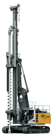
Max. drilling depth 16.3 m with auger cleaner, without Kelly extension Max. drilling depth 20.3 m with auger cleaner and Kelly extension
