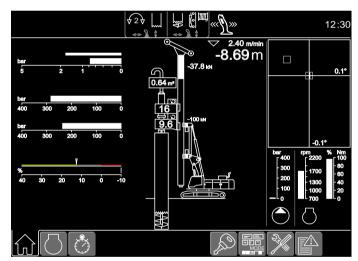
Display for double rotary drilling
