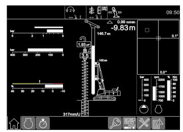
Display for continuous flight auger drilling
