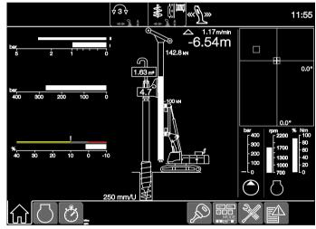
Display for full displacement drilling
