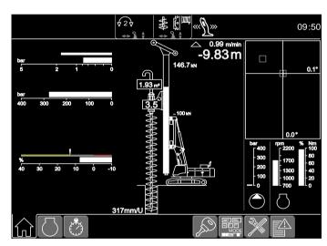
Display for continuous flight auger drilling
