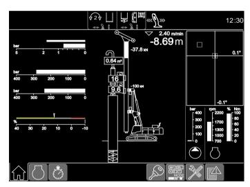
Display for double rotary drilling
