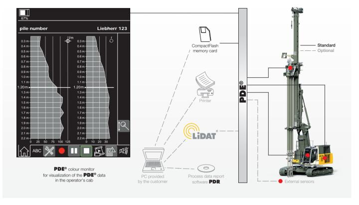
Depending on the application the recorded and processed data are displayed on the PDE® touchscreen in the operator's cab, e.g. in the form of an online cast-in-place pile.
