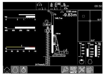
Display for continuous flight auger drilling
