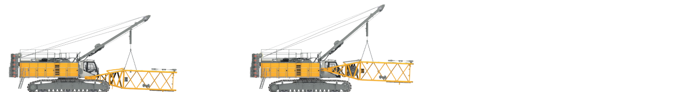
Assembly of boom foot
